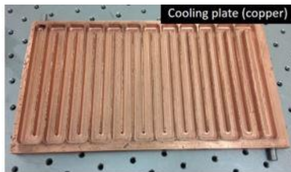
Figure 2 Copper plate used to circulate cold water on the cold surface
