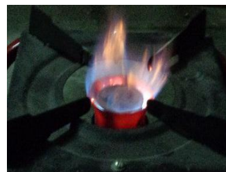
Figure 2: Pictorial view of the free flame in conventional cooking kerosene stove
