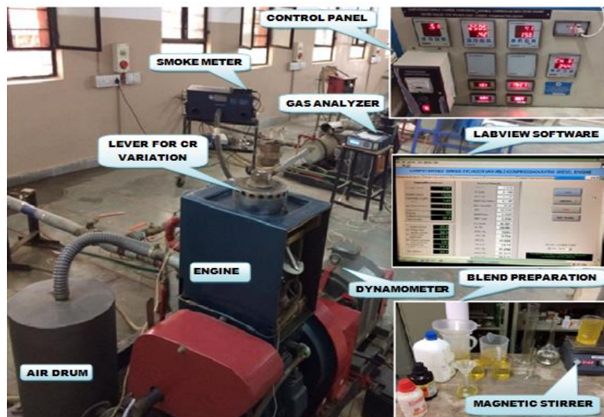
Figure 3. A pictorial view of the experimental setup
