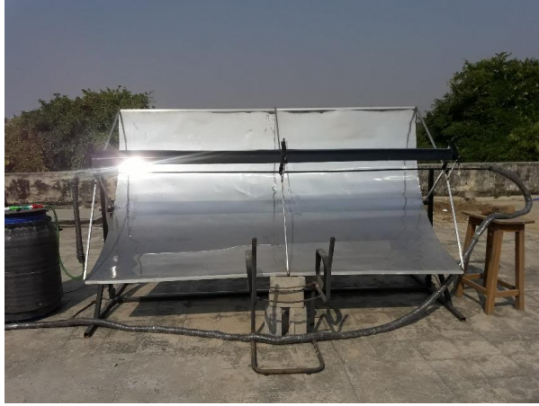
FIGURE 2. EXPERIMENTAL SET-UP WITH SECONDARY REFLECTOR
