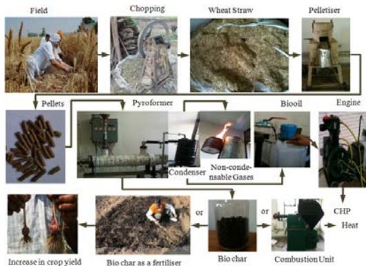
Figure 1 Intermediate Pyrolysis process using wheat straw
