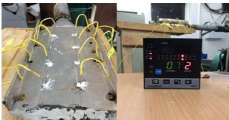
FIGURE 3. TEMPERATURE MEASUREMENT SETUP
