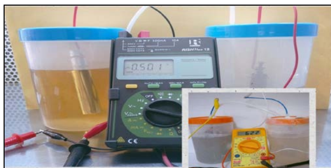
FIGURE 3. Setup of Salt Bridge Based MFC
