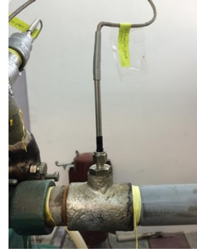
FIGURE 4. INLET TEMPERATURE MEASUREMENT THERMOCOUPLE
